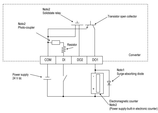
Figure 5.3 Electromagnetic Counter Connection Example
